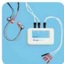
AR-279201-Kit Multi-RIP Inductive Interface module w/SUM Channel *Kit includes SUM Module (# AR-279201 ) abdomen wireset (# PS AR-279202 ), chest wireset (# PS AR-279203 ), and SUM/output wireset (# PS AR-279204 ). Connects to any SleepSense Inductive Band – AAA Batteries.
